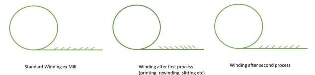
It's good to remember that every time the paper is processed after this (eg rewinding or slitting), the peel direction will be reversed. So, if initial trials are performed on unprinted paper but actual production will use printed paper, take care with the peel direction.
