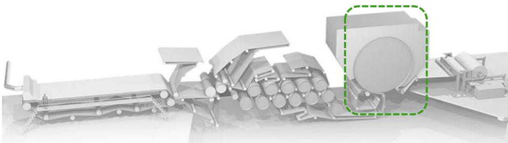
*(MG machine with the MG cylinder marked in green)*
