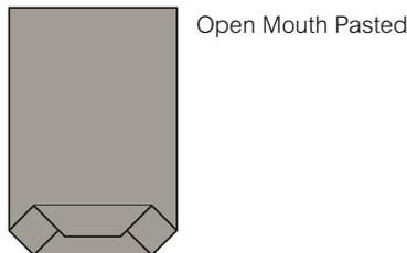
These result in greater stability of the filled sacks on conveyors during top closure and also present a good flat area for the addition of extra identification data.
