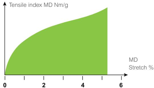
This diagram shows that TEA is the combination of tensile strength and stretch. The TEA is the coloured area under the curve.
