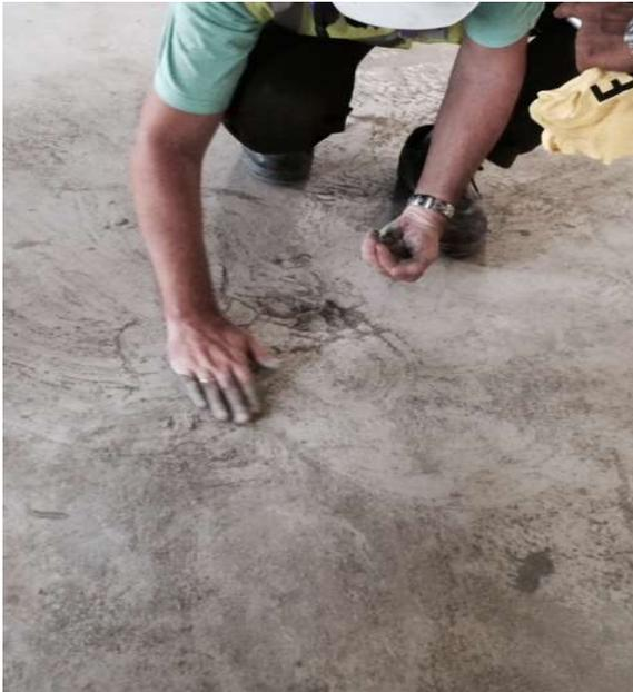
*Cement loss after the drop test of WPP sacks in India.*
